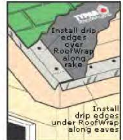
Installing drip edges
